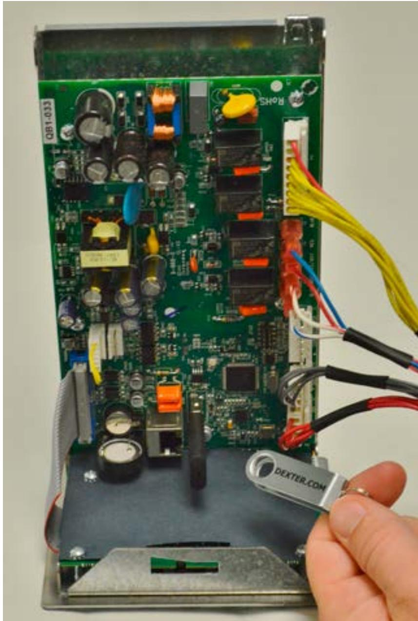
**C.** Once the program is uploaded successfully the control will scroll "DONE REMOVE USB". The USB drive can be safely removed at this point.
